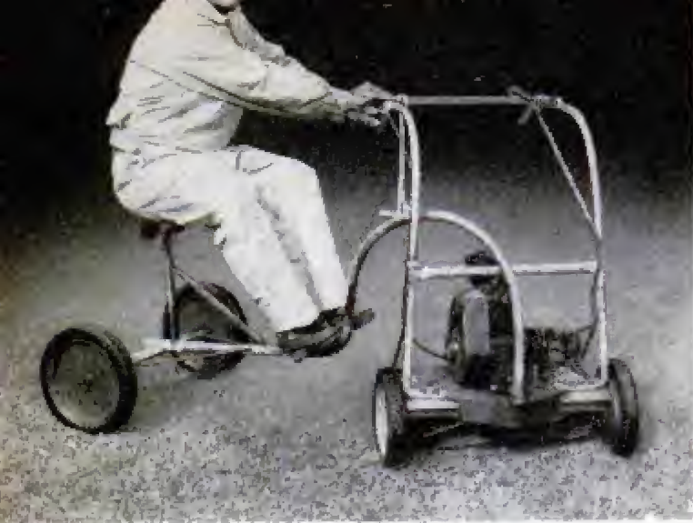
The lawn mower-trailer unit can be made to turn in its own length, an essential feature when mowing around flower beds and in irregularly shaped plots
